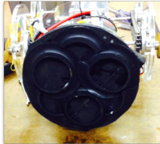
The RC components were contained using velcro, and the wires were contained with zip ties. Unfortunately the zip ties limited our movement. One other issue we ran into was that the hardware in the chassis would vibrate out of its sockets over time, so we added lock washers to every 4-40 screw.
