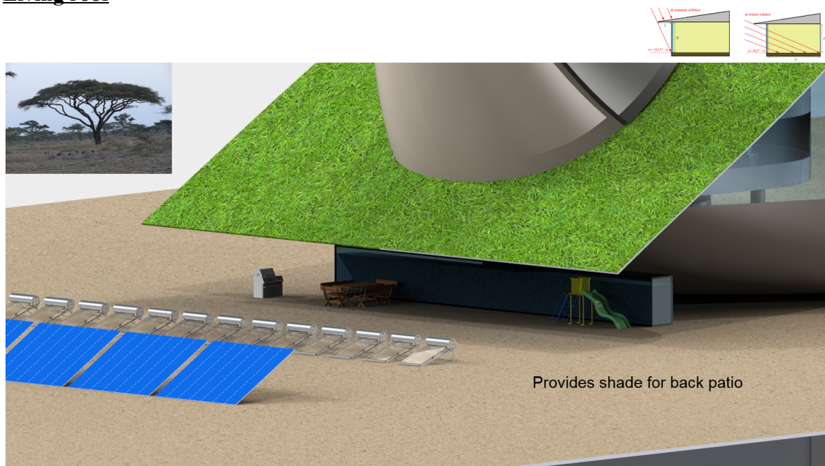
Figure 4. Living roof angled toward the south, provides more shading for the structure.
