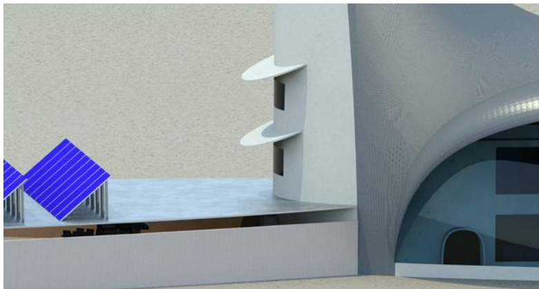
Figure 26. Close-up view of window overhangs, with realistic depiction of sun angle.
